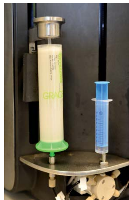
Left: the Flash cartridge by Grace (silica 40 micrometer) that can withstand a maximum pressure of 200 psi.
