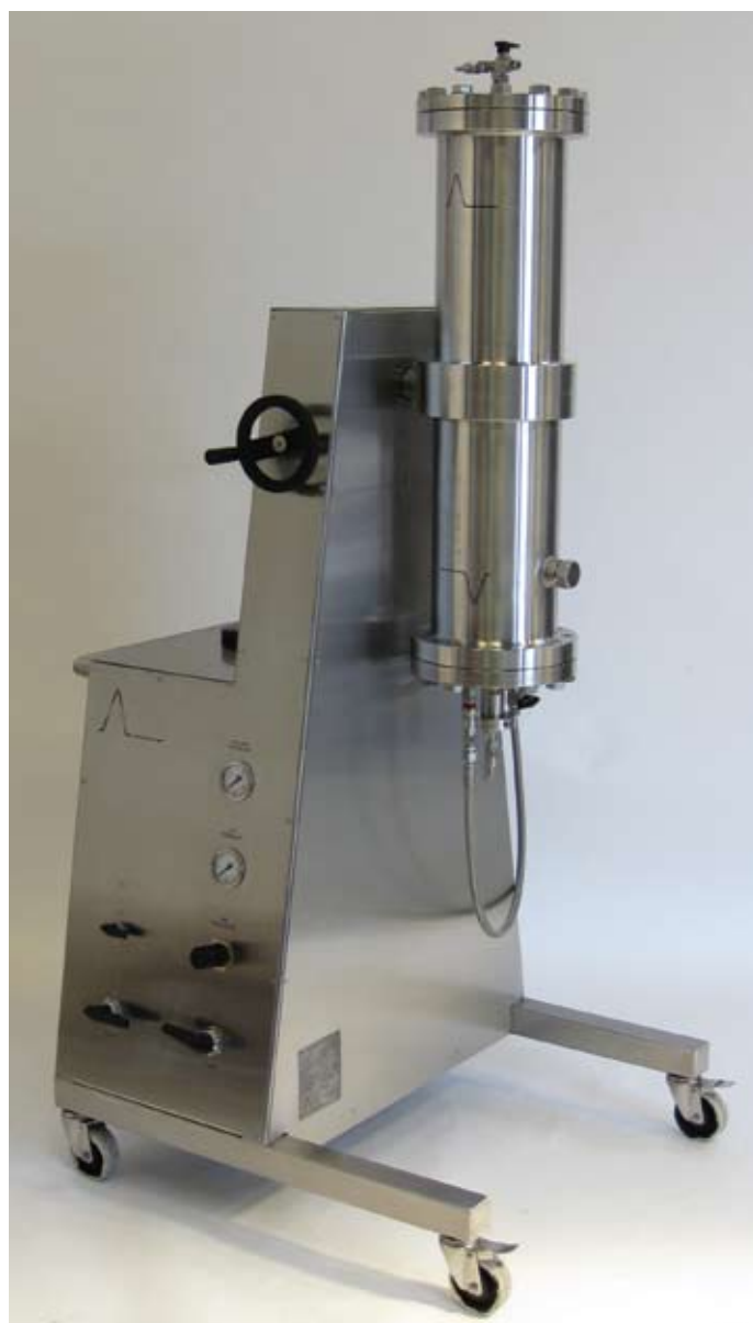
The 200mm x 700mm HPLC column is a slim, mobile construction. It fits to a lab door of 800mm width. Mechanical column turning device included to facilitate packing and unpacking. All Peak Biotech A/S columns are custom designed to meet exactly the customer needs.
