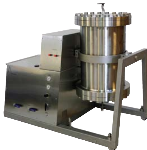
600mm x 1200mm HPLC column. Pressure rated for up to 100 bar. Mobile construction with motor driven column turner to facilitate column packing and unpacking.
