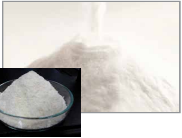
Figure 1. Miglyol loaded on Syloid® 244 FP silica results in a free-flowing powder with oil adsorption of 1:2.5 (Syloid® 244 FP silica:Oil).
